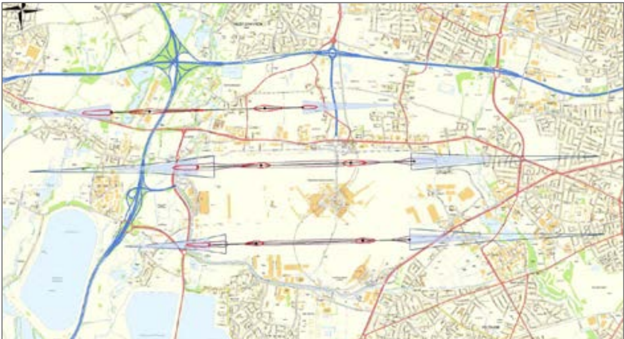
Figure 3.18: Future public safety zones at Heathrow
