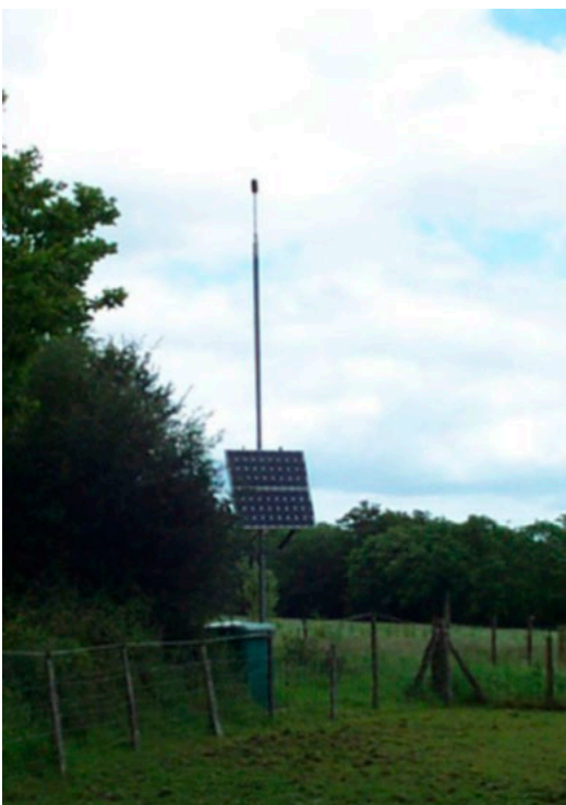
Figure 19: Noise monitoring terminal
